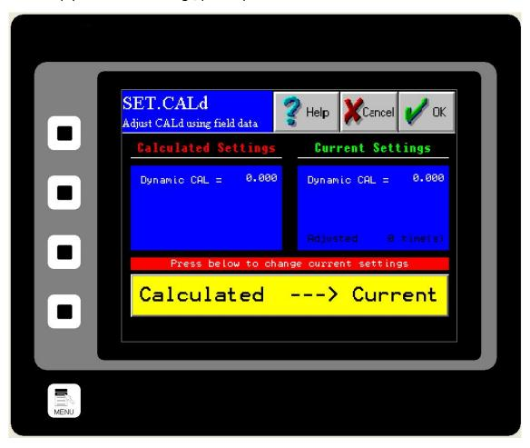
**Step 11:** To accept the new Dynamic Calibration press the YELLOW CACULATED to CURRENT Button and press the OK Button. A pop up screen will appear, asking if you are sure you would like to accept this value. Press YES.
